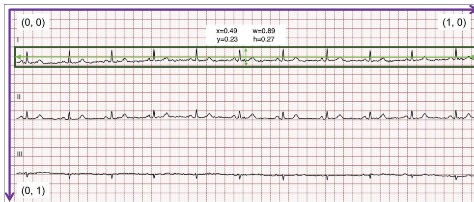
Figure 5: Illustration of the YOLO bounding box format, which includes the class ID, normalized center coordinates (x, y), and the bounding box width and height (w, h), all expressed relative to the image dimensions
