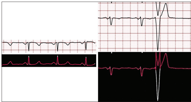
Figure 7: Digitization performance using the method from Fortune et al. [18] on our single-lead ECG dataset. Top: input single-lead ECG images. Bottom: extracted signals (red) overlaid on original images. Left: example from the normal dataset; Right: example from the overlapping dataset
