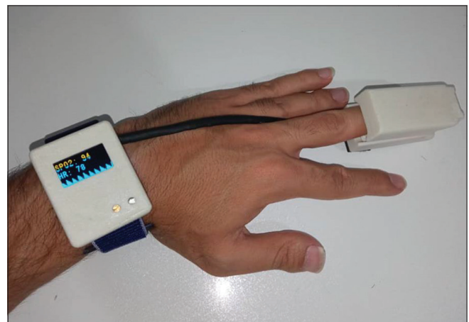
Figure 5: Picture of the implemented patient wristband: (a) wristband and (b) pulse oximeter sensor probe
