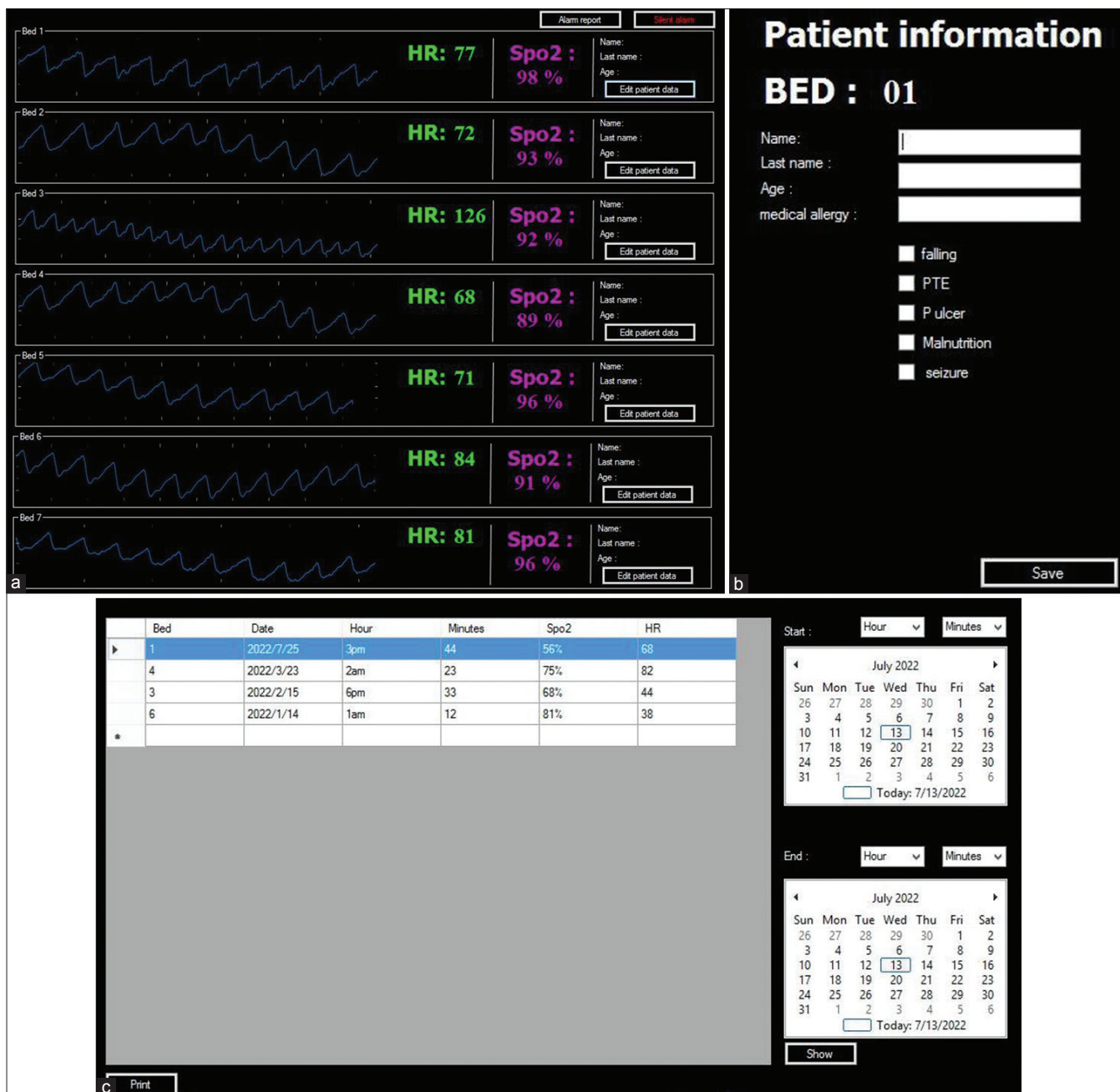
Figure 4: Proposed central GUI software: (a) main page, (b) page dedicated to patient identity information editing, and (c) page dedicated to history of the emergency conditions. GUI – Graphical user interface
