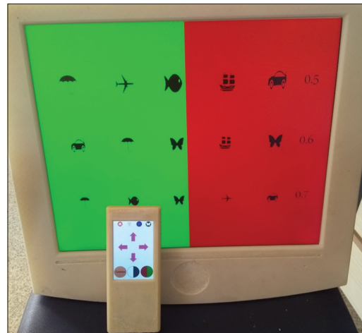
Figure 8: The implemented VAM system. VAM: Visual acuity measurement
