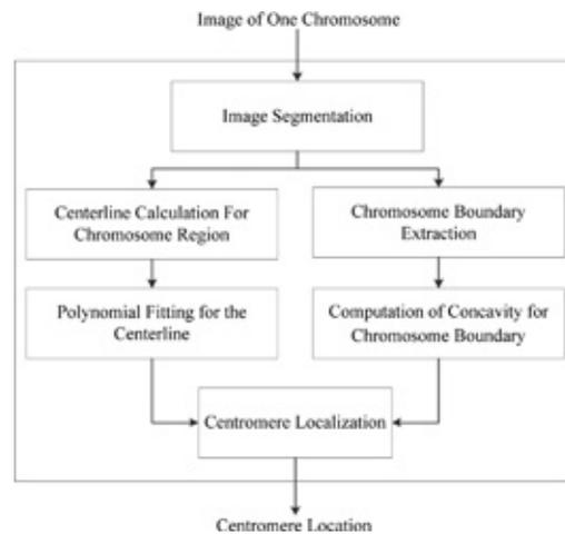
**Figure 2:** Block diagram of the proposed algorithm for centromere localization
