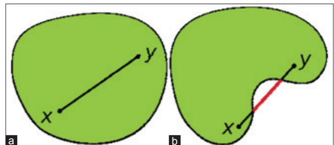
Figure 6: Demonstration of convex and nonconvex regions, (a) in a convex region, for every pair of points within the region, every point on the straight line segment that joins them is also within the region, (b) in a nonconvex region, previous condition is not valid for some pair of points<sup>[15]</sup>
