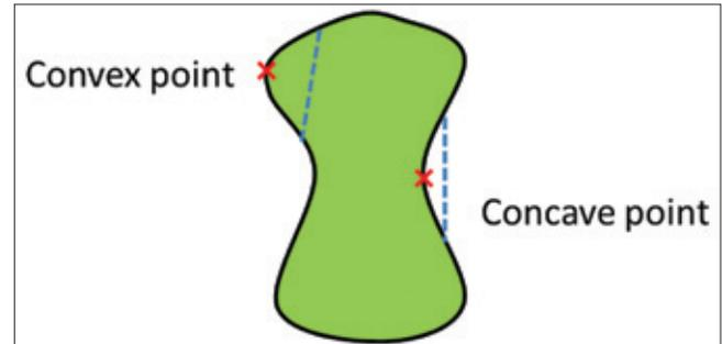
Figure 7: Illustration of concave and convex points
