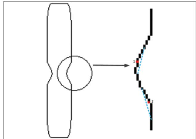
Figure 8: Demonstration of the proposed method to computation of concavity degrees of two pixels. For pixel 1, which is a concave point, the corresponding line (that connects two pixels by  $h$  distance before and after it) has no intersection by the region. On the other hand, for pixel 2, which is a convex point, all of the corresponding line overlies on the region
