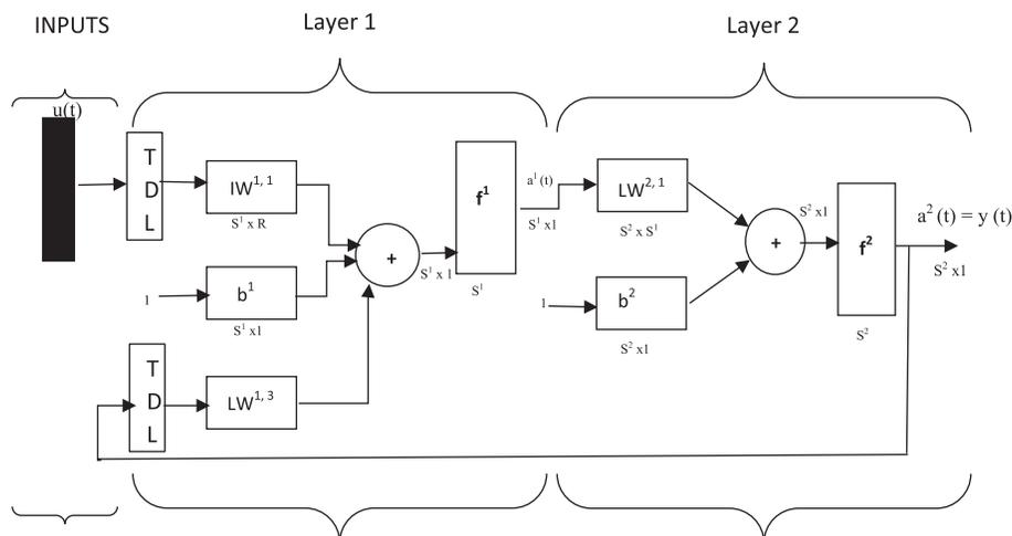
Figure 1: Two-layer NARX network structure with  $s$  outputs<sup>[21]</sup>
