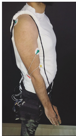
Figure 2: Prototype attached to the human body. The bag is strapped to the thigh and waist. Heart rate and oxygen saturation sensor are attached to the forefinger. Electromyography electrodes are placed over the biceps muscle, and an accelerometer is located on the back or around the chest
