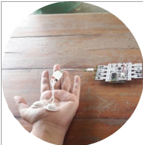
Figure 1: Electrode placement of electrodermal activity sensor
