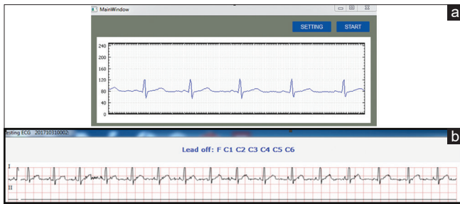
Figure 14: (a) Electrocardiogram waveform from proposed device (b) electrocardiogram waveform from EDAN electrocardiogram
