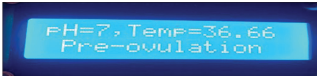
Figure 5: The designed device display that the woman is in preovulation phase with a potential of hydrogen = 7 and a Basal Body Temperature (BBT) = 36.66°C
