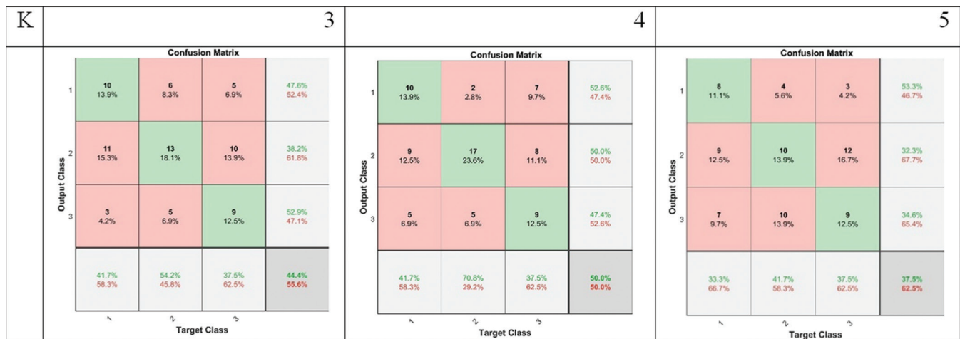
Figure 15: Confusion matrix for classifying using the root-mean-square value of the signal in the seventh window
