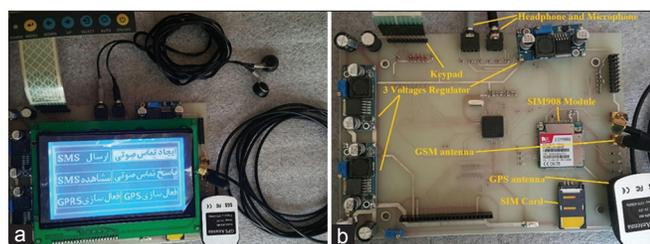
Figure 2: Complete simple version of automatic vehicle location board with SIM908 Module and LCD in (a). Annotated board without LCD is shown in (b)
