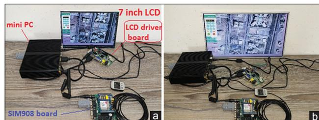
Figure 4: Complete automatic vehicle location board with SIM908 Module in advanced version is shown with two sizes of LCD. (a) 7-inch LCD (b) 15.6-inch LCD
