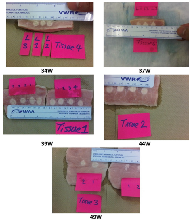
Figure 1: Tissue slices revealing high-intensity focused ultrasound lesions in their middle parts at acoustic powers of 34, 37, 39, 44 and 49 W
