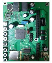
Figure 6: ARM-based microcontroller evaluation board
