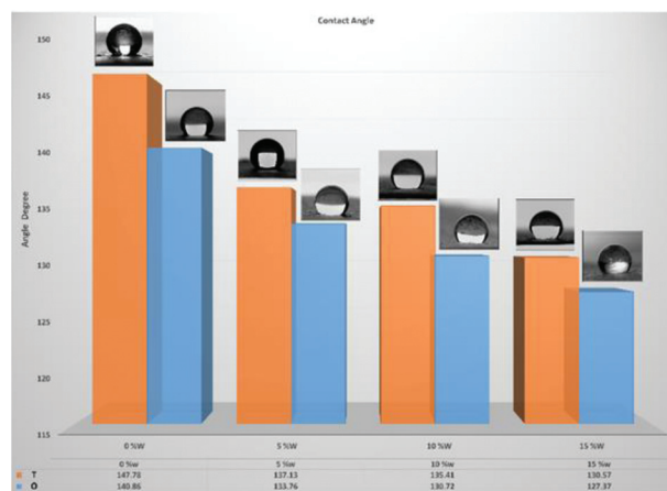
Figure 10: Wettability result (contact angle) of sample containing 0, 5, 10, and 15% lignin in PCL scaffold
