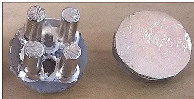
**Figure 1: Gold coated dry multipin electrode for electroencephalogram recording through the hairs and dry flat electrode for electrocardiogram or forehead-electroencephalogram recording. The electrode's base had a diameter of about 11 mm**
