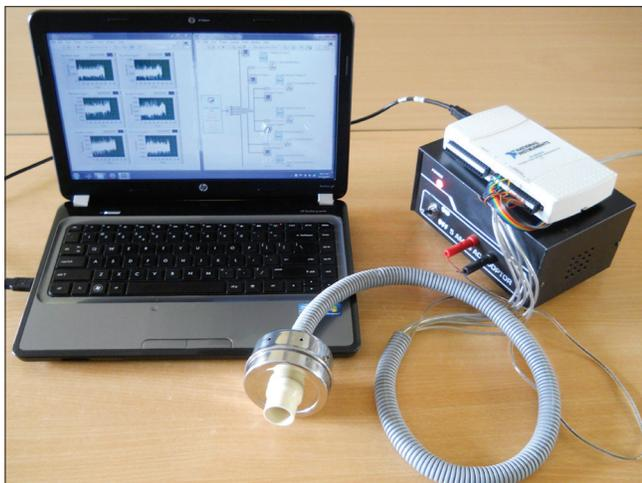
Figure 1: Electronic-nose system using data acquisition card
