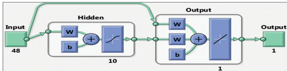
Figure 5: Network diagram of single-layer cascade-forward neural network classifiers
