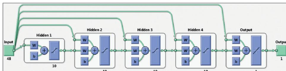
Figure 6: Network diagram of multilayer cascade-forward neural network classifiers
