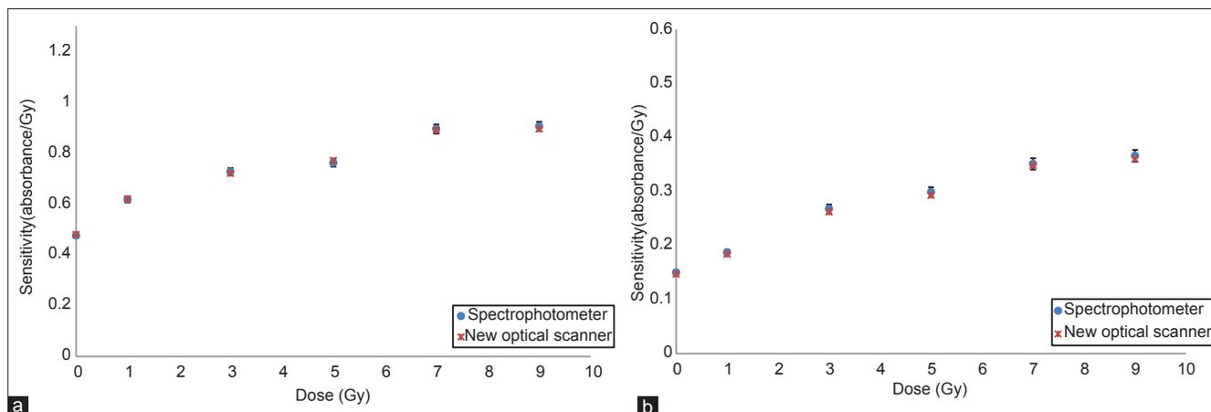
**Graph 2a:** Comparison between optical dose-response curves of the polymer gel samples measured by the new Optical scanner and Spectrophotometer systems. (a) NIPAM sample (with 2% error bars) Graph 2b: Comparison between optical dose-response curves of the polymer gel samples measured by the new Optical scanner and Spectrophotometersystems. (b) PAGAT sample (with 3% error bars)
