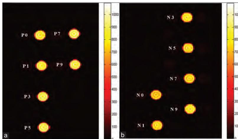
**Figure 4:**  $T_2$ -weighted image of the gel samples with different absorbed dose values. The absorbed dose values are ranging from 0 to 9 Gy. (a) PAGAT gel samples. P 0 is used instead of the PAGAT sample that was irradiated to 0 Gy similar to other samples. (b) NIPAM gel samples. N 0 is also used instead of the NIPAM sample that was irradiated to 0 Gy similar to other samples
