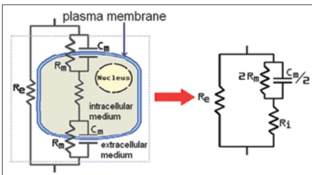
Figure 3: A cell equivalent circuit<sup>[1]</sup>
