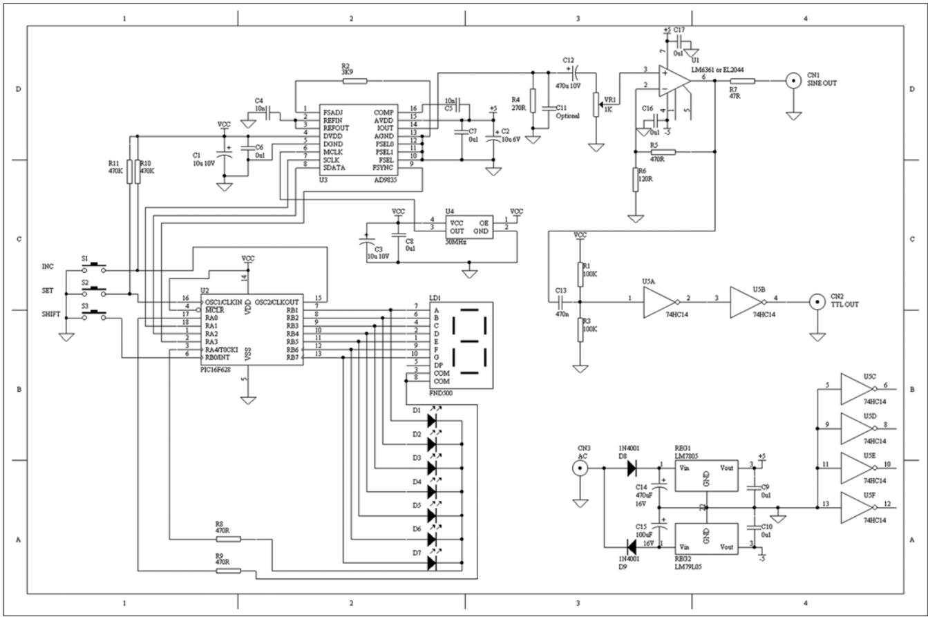
Figure 6: Schematic of designed direct digital synthesizer
