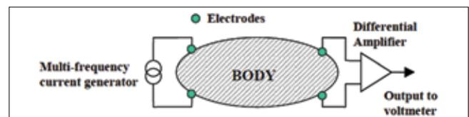
Figure 4: General design of bioimpedance measuring device<sup>[3]</sup>
