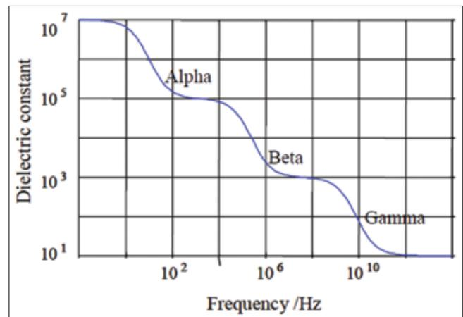
Figure 2: Decrease in dielectric constant with frequency<sup>[3]</sup>
