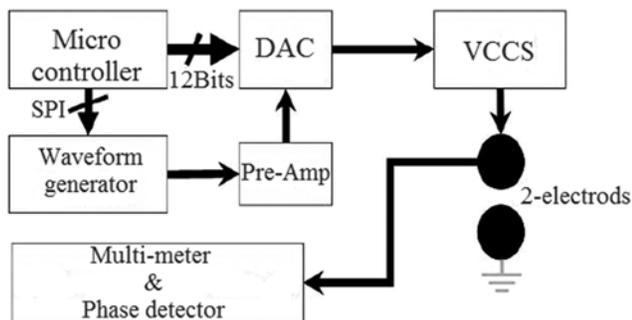
Figure 7: Proposed design block diagram<sup>[14]</sup>
