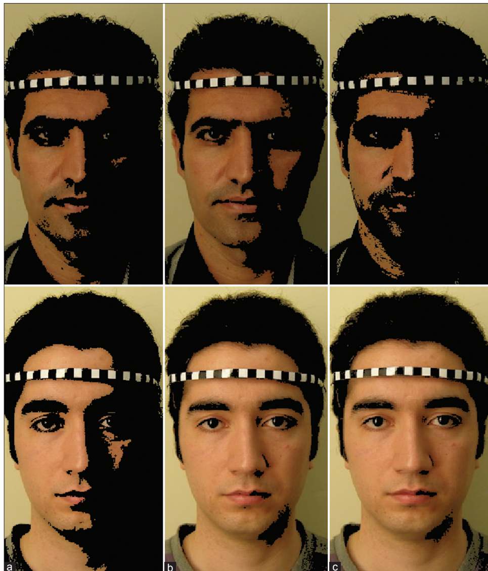
Figure 3: (a) Segmented image based on Otsu thresholding using BFO, (b) segmented image based on Kapur thresholding using BFO, (c) segmented image based on Kapur thresholding using genetic algorithm
