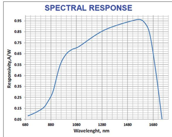
Figure 26: The spectral response of the receiver<sup>[30]</sup>
